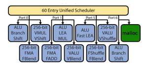
A small, dedicated, software-managed malloc cache can speed up allocation by 30%, with only 0.006% area overheads.
