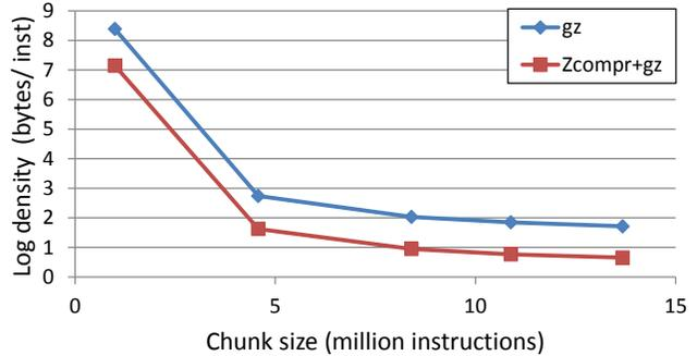
Figure 10. Effect of log chunk size on compressed log density for the Linux 2.6 workload.
