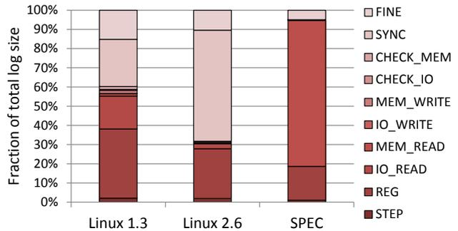
Figure 8. Distribution of trace commands in logs compressed using our scheme. Unpredictable commands take up 75% of final size.
