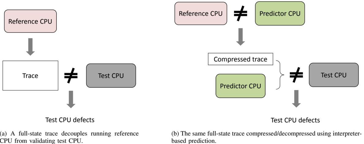
Figure 1. Sample co-simulation workflow that validates a *test CPU* model against a *reference CPU*.
