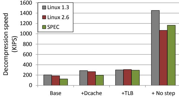
Figure 11. The effect of dedicated optimizations targeting decompression speed. The last three sets of bars represent incrementally enabling the three optimizations described.
