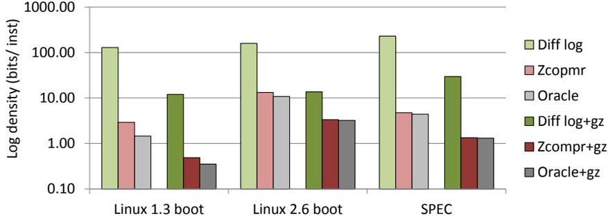
Figure 7. Log density in the compressed logs. Light bars show single-stage compression, while darker ones use gzip as a second stage compressor. Bars marked as *oracle* use a fully-functional CPU model that is able to achieve virtually perfect prediction.
