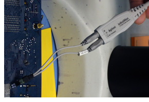
(b) Sensing voltage using an InfiniiMax 1.5GHz 1130A differential probe that has ultra low loading.
